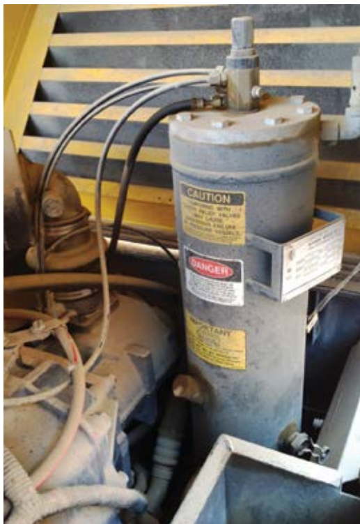
Fig. 1: Due to high compressor pressure, filter/separators are contained within a vertical steel tank near the compressor head unit
