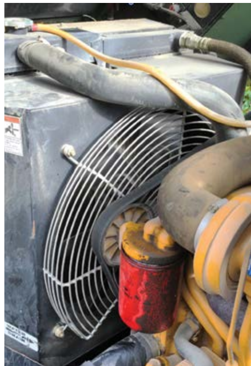
Fig. 2: A cooling fan forces fresh air through the engine's radiator and various heat exchangers
